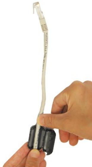
3. Loop the cable around and through the core. This helps "lock" the core in place, and may be required in circumstances with severe interference.
