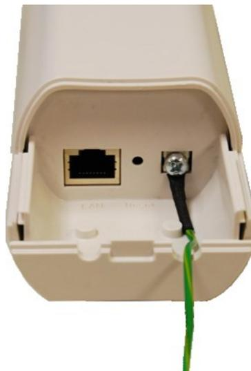
3. Connect the grounding wire to earth ground.
