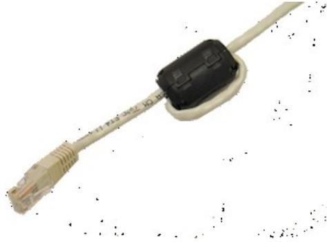
5. Connect the Ethernet cable with suppression core to the “Data In” port of the PoE injector.
